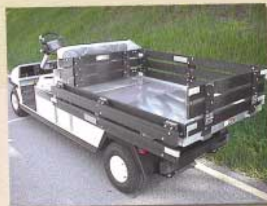
Stake side kits let you haul trash and trimmings with ease. (Carryall 6 pictured with hinged modifications.)
