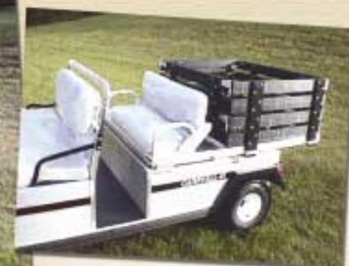
This Carryall 6 has a middle seat that flips forward for extra cargo space (SVP112501).
