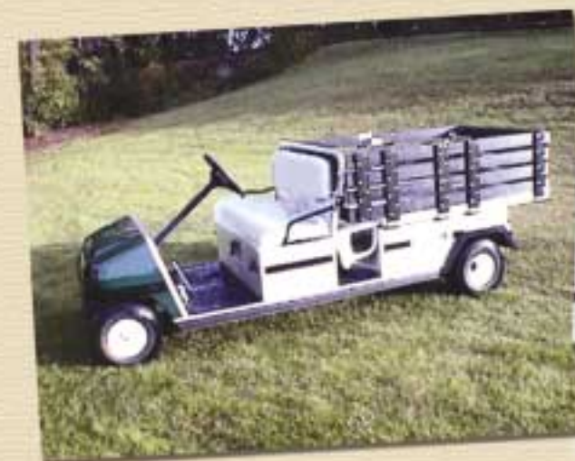
This Carryall 6 has a middle seat that flips forward for extra cargo space (SVP112501).
