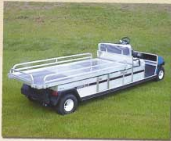
Increase the efficiency of your Carryall 6 XL with a longer bed (SVP107701) and drop-down rails.
