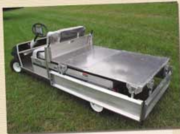
Provide access for a forklift or simply add comfort with a fold-down cargo box (Carryall 6 shown with SVP210701).
