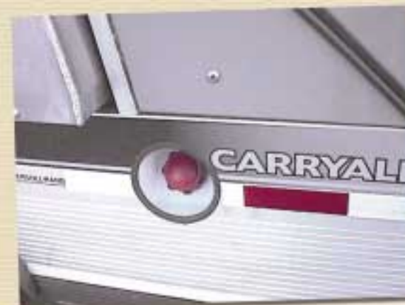
An external fuel fill installation makes refueling quick and easy. (Carryall 2, SVP180201, or Carryall 6, SVP208701.)
